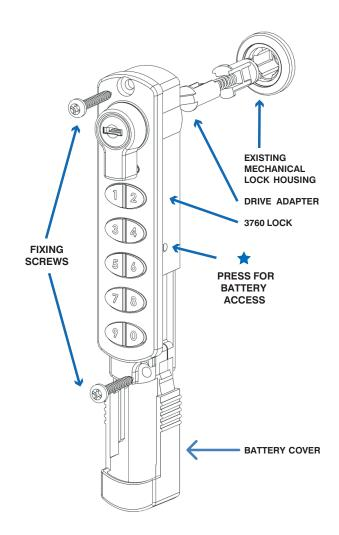
BATTERY COVER IS REMOVED BY INSERTING A PAPER CLIP OR SIMILAR INTO THE HOLE MARKED AND SLIDING COVER AS SHOWN
